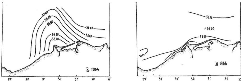
Fig. 3 — Surface salinity distribution off the mouth of the Nile River before the Aswan High Dam (October 1964) and after completion of the High Dam (November 1966).
