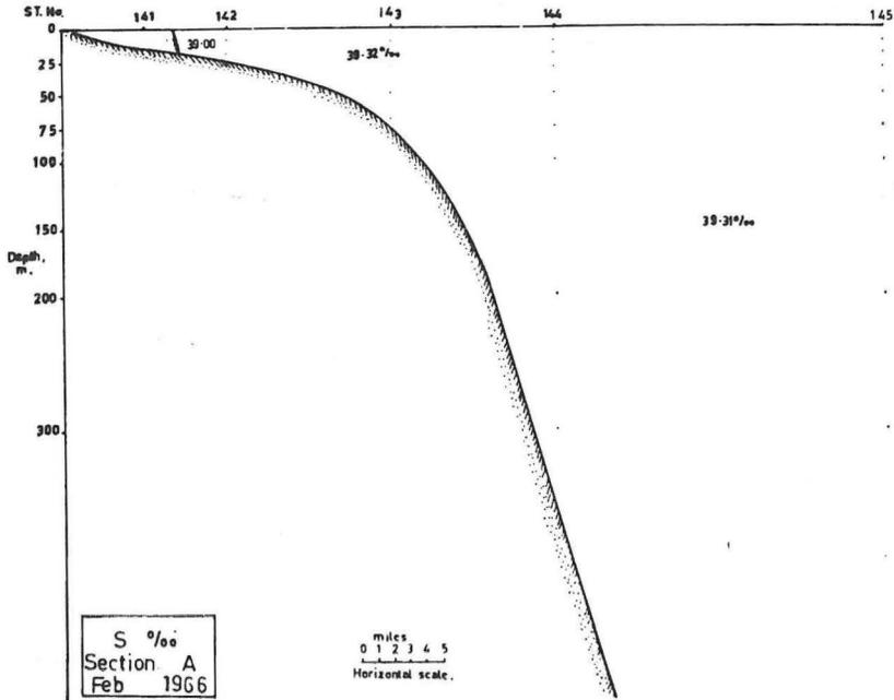
Fig. 4a — Vertical distribution of salinity in Section A, El-Arish, Sinai (Long. 33°40') in February 1966.
