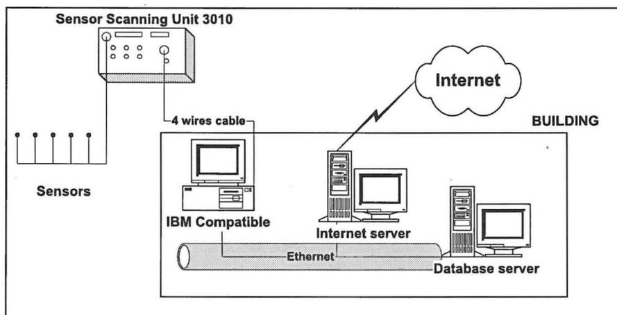
Fig. 2. Scheme of the AANDERAA Instruments Sensor Scanning Unit connection to the local area network (LAN)
