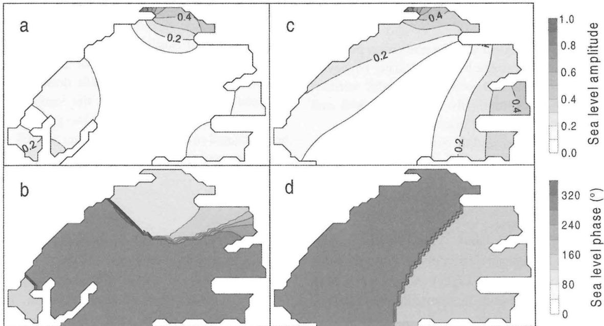
Fig. 6. The distributions calculated for the 3.0-min mode of (a) relative sea level amplitude and (b) phase for the run with the marina, and (c) relative sea level amplitude and (d) phase without the marina. The value of 1.0 equals 4.5 cm for the run with marina and 13.5 cm for the run without marina
