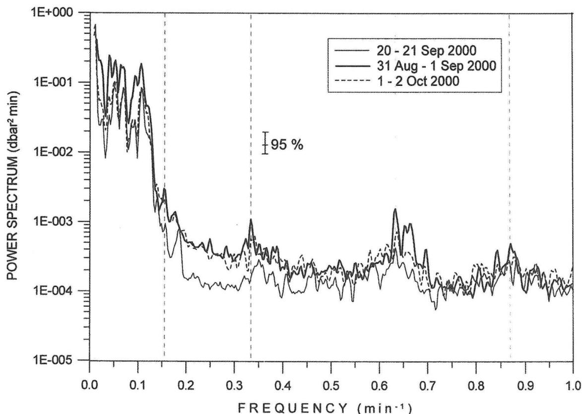
Fig. 2. Bottom pressure (sea level) power spectrum calculated for the periods 31 August-1 September, 20-21 September and 1-2 October 2000 (40 degrees of freedom). Vertical dashed lines indicate seiche periods
