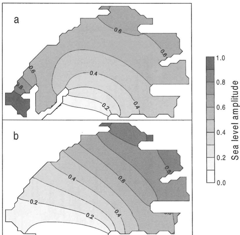
Fig. 4. The distributions of first-mode relative sea level amplitude calculated for the runs (a) with and (b) without the marina. The value of 1.0 equals 16.0 and 16.5 cm for the first and the second run, respectively
