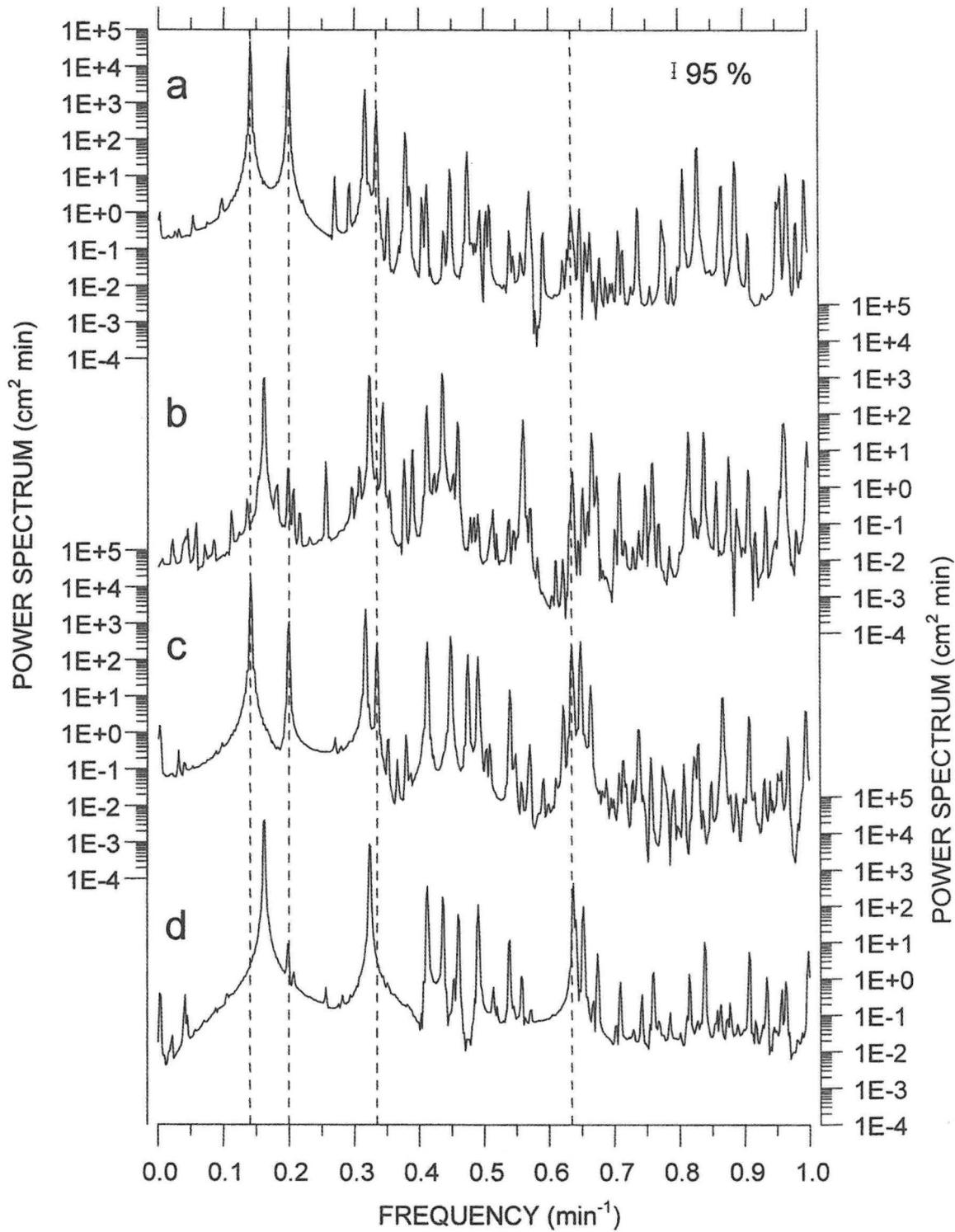
Fig. 3. Power spectra of the sea level displacements modelled at the P1 station (a) with and (b) without nautical marina, and at the P2 station (c) with and (d) without the marina. Dashed lines indicate seiche periods of 7.1, 5.0, 3.0 and 1.6 min
