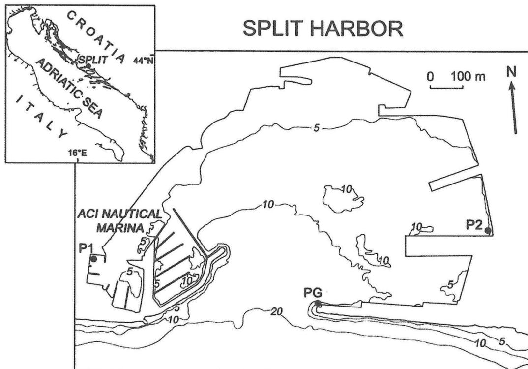
Fig. 1. Bathymetry (in m) of the Split harbor with position of the pressure gauge (PG), and locations P1 and P2 where the modelled sea level spectra are computed
