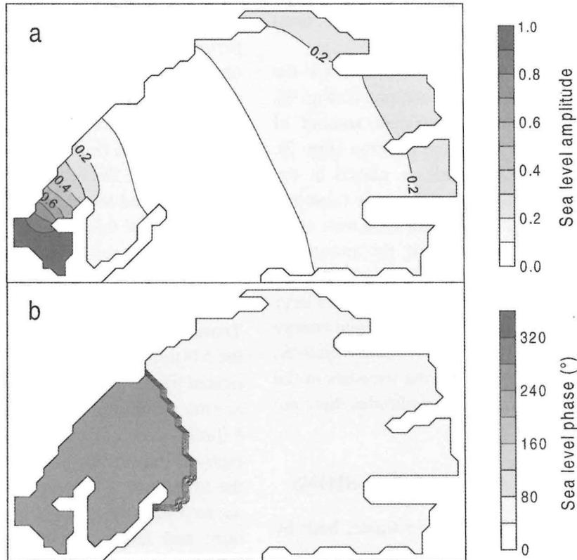
Fig. 5. The distributions calculated for the 5.0-min mode of (a) relative sea level amplitude and (b) phase for the model run with the marina. The value of 1.0 equals 10.0 cm
